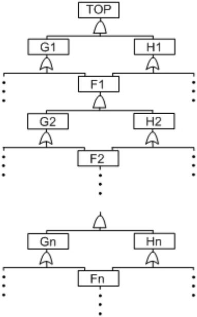
**Figure 6.** A fault tree with  $2^n$  paths from TOP to  $F_n$ .
