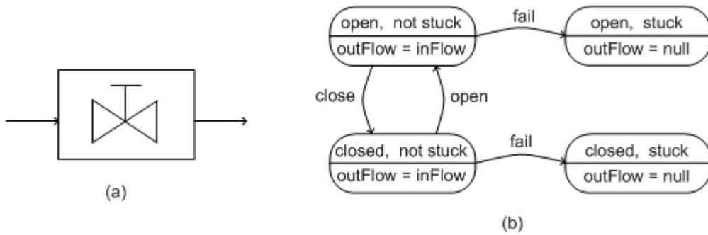
**Figure 1.** A valve and the mode automaton that describes it.
