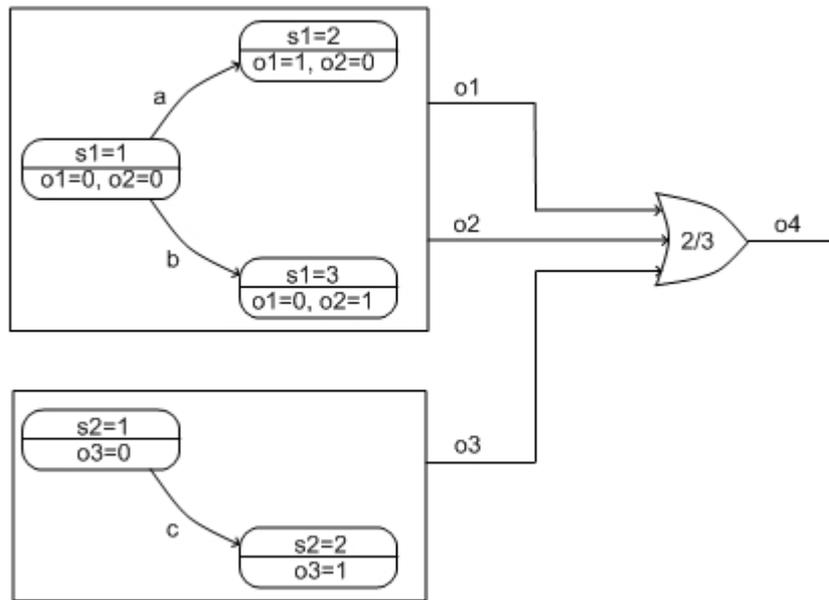
**Figure 3.** A mode automaton that causes non coherency of fault trees
